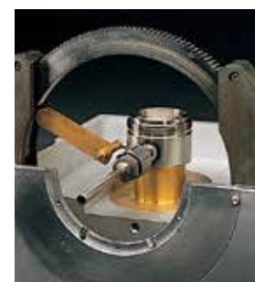
▲ Automated Welding System
